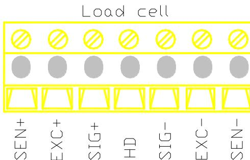
1. The exciting voltage for the load cell is 5VDC, the largest output current 120mA, maximum connect 6 pcs 350Ω load cell;
